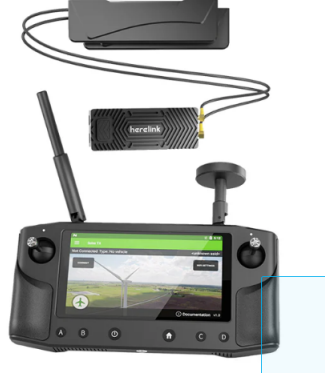
Figure 20: The HereLink GCS Kit
